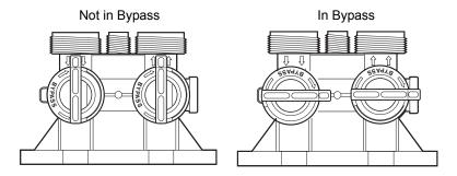
Figure 4 Autotrol Series 256 Bypass Valve
